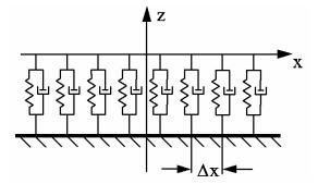
Fig. 1 Equivalent one-dimensional visco-elastic foundation
