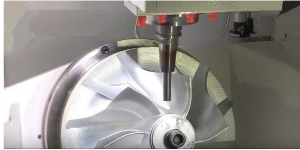
Fig. 9 The 5-axis milling operation of test impeller
