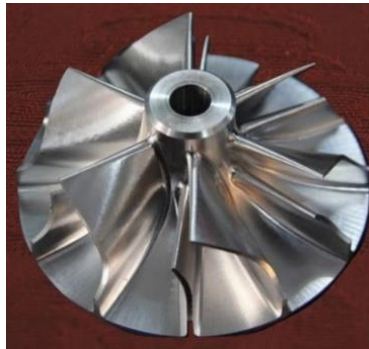
Fig. 10 The real machined AL impeller
