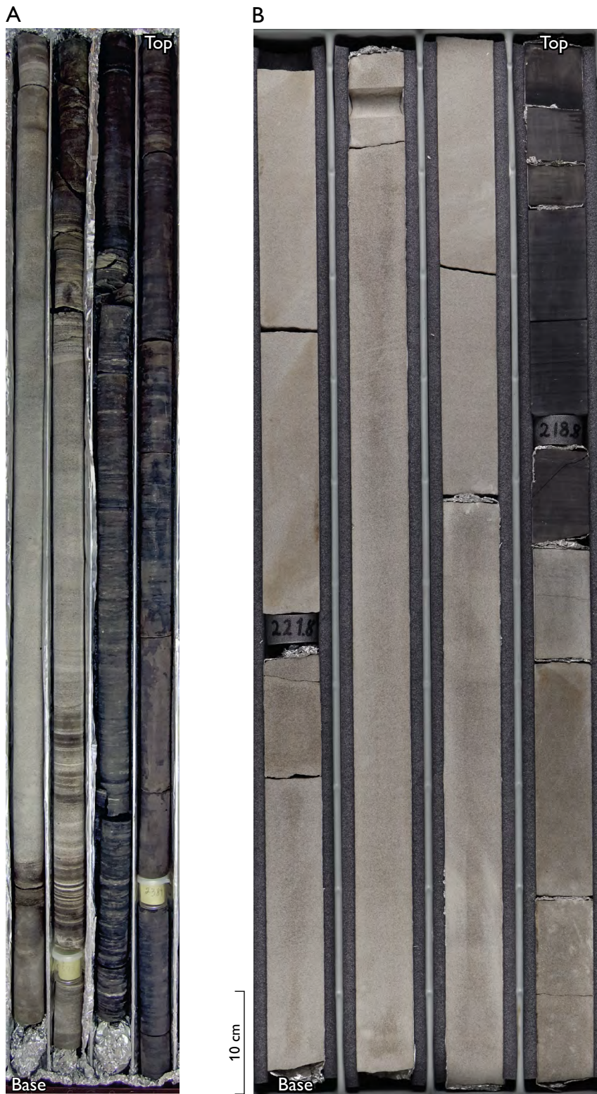
Fig. 10. Core photographs from the middle Oxfordian C. tenuiserratum Chronozone. A: Slope facies from the Lollandselev-2 borehole (26.75–22.75 m) comprising laminated and massive gravity-flow sandstones overlain by mid-dark grey biomottled silty and sandy mudstone. B: Basin-floor facies from the Blokselev-1 borehole (222.07–218.25 m) consisting of massive, structureless gravity-flow sandstones overlain by laminated very dark grey to black mudstone.
