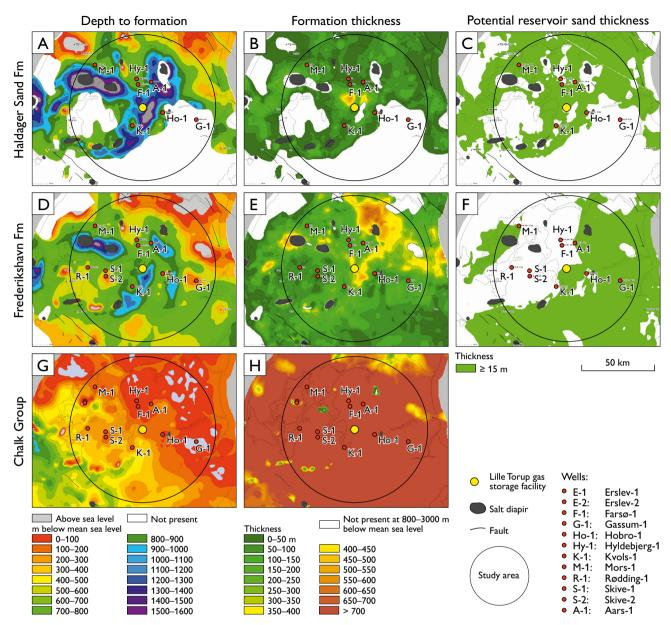
Fig. 3. WebGIS-generated maps of potential brine storage formations in the study area. Reservoir quality is assessed based on depth to formation top, formation thickness and potential reservoir sand thickness.
