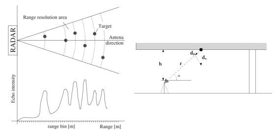
Figure 1: Radar range resolution principle (left) and radial displacement and projected displacement (right)
