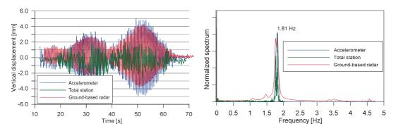
Figure 5: Displacements (left) and periodogram (right) during jumping-centre of the structure
