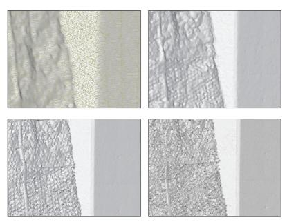
Figure 5: Level of detail of cloud of points shown as shaded cloud of points, detail from left: low, medium, high, ultra high (down)
