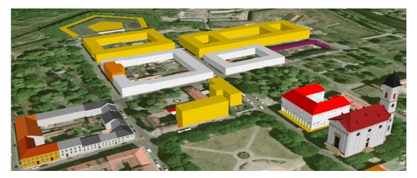
Figure 7: View-dependent visualization of different LODs of buildings in Terezín (adopted from Janečka et al. (2013)).
