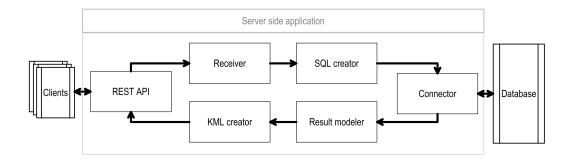
Figure 2: Designed schema of server-side part of application
