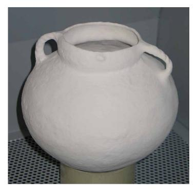
Figure 14: The final model created by 3D printer Zprint 450 (after editing in Geomagic software)
