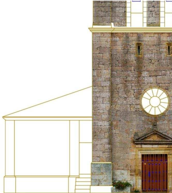
Figure 8: Photo grinding walls in the tower of the Santa Marina's church in Villadiego, Spain.
