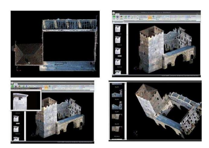
Figure 3: 3D point cloud models with RGB information
