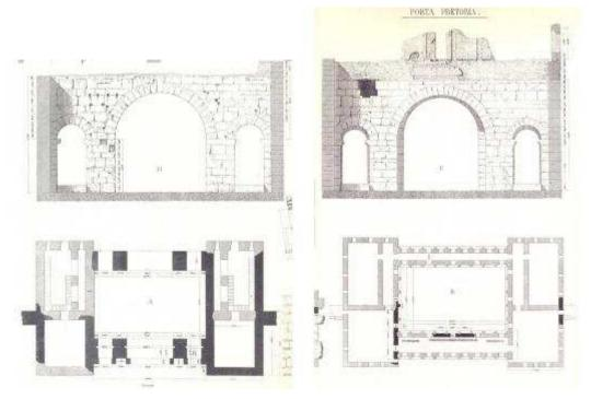
Figure 1: Praetorian Gate, plans and elevations in the reconstruction of Carlo Promis (Tav. V)
