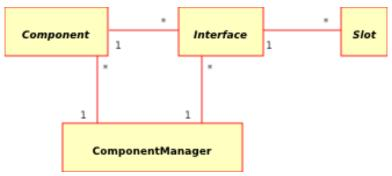
Figure 3: Class diagram of component architecture.
