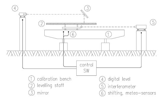
Figure 1: Scheme of horizontal comparator for system calibration
