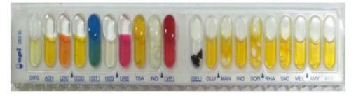
Figure 1: API 20E system for characterization of K. pneumoniae
