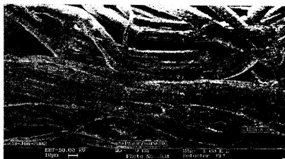
Fig.4 Scanning electron micrograph of Flax-g-poly(MMA)
