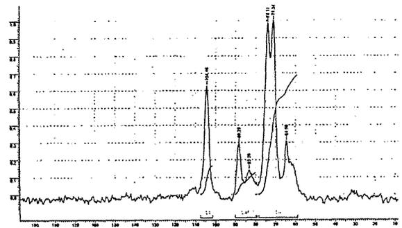
Fig.1 <sup>13</sup>C Solid-state NMR of Raw Flax
