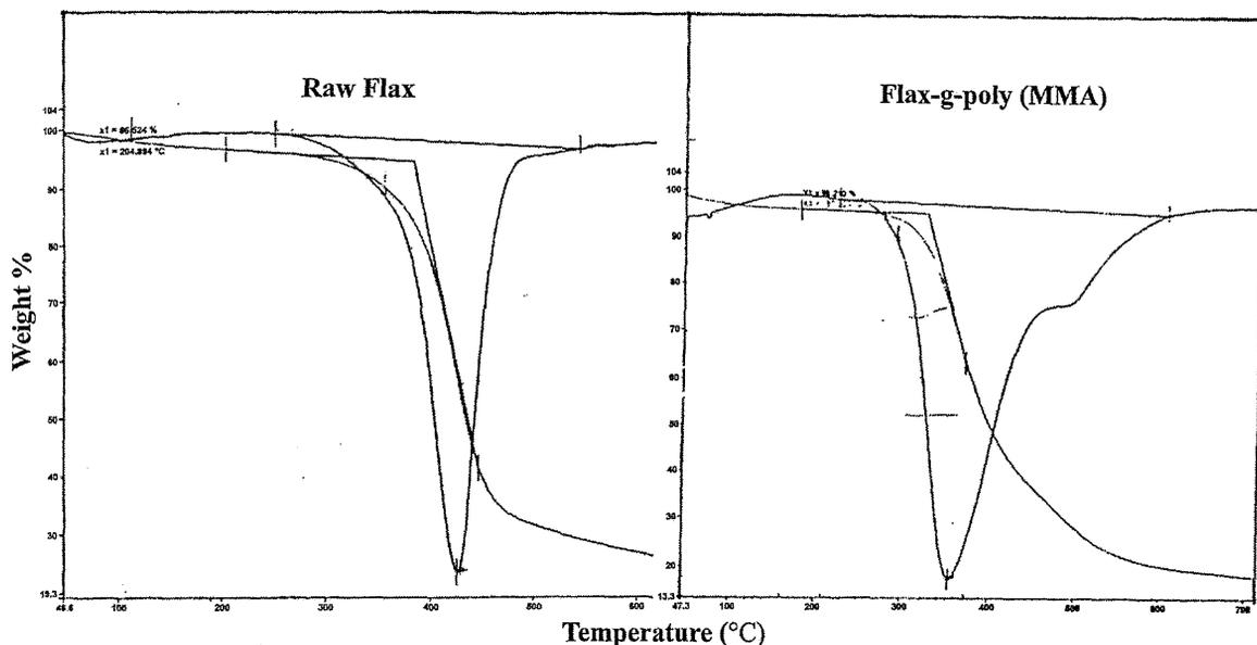
Fig.7 TG curves of flax and flax-g-poly (MMA) (Sample 14 of Table I)
