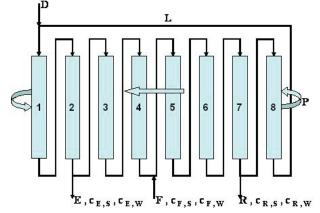
*Fig. 2.:* One of the applied practical solutions of the Simulated Moving Bed
