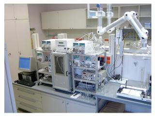
Fig. 4.: KNAUER CSEP 9116 SMB unit assembled for quasi-continuous process
