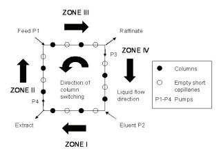
*Fig. 1:* Conventional four-zone SMB unit with eight columns
