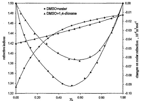
Fig.2 Refractive indices and changes of molar refraction on mixing vs. mole fraction of DMSO. Binary systems at T=298.15 K.
