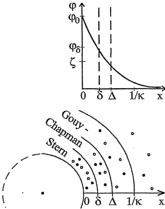
Fig.1 Scheme of electric layer and adherent electrical potential
