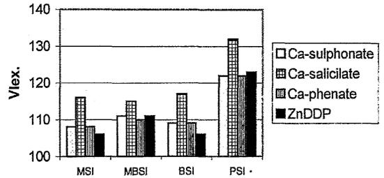
Fig.3 Changes of viscosity indexes (VIex) of the additive blends
