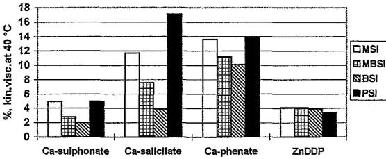
Fig.2 Relative changes of kinematic viscosity at 40 °C by the interactions of the additives
