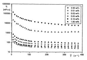
Fig.8 Apparent viscosity (η) vs. shear rate ( Υ ) flow curves for the 77.5 wt% alumina + sodium polyphosphate suspensions studied.
