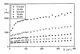
Fig.1 Shear stress ( $\tau$ ) vs. shear rate ( $\dot{\gamma}$ ) flow curves for the alumina suspensions studied.
