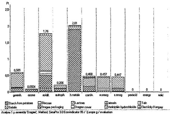
Fig.1 Evaluation histogram for dragee production
