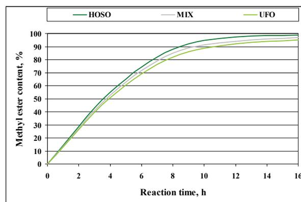
Figure 1: Methyl ester content of products as a function of transesterification time (catalyst *Candida antarctica* (Novozym 435))
