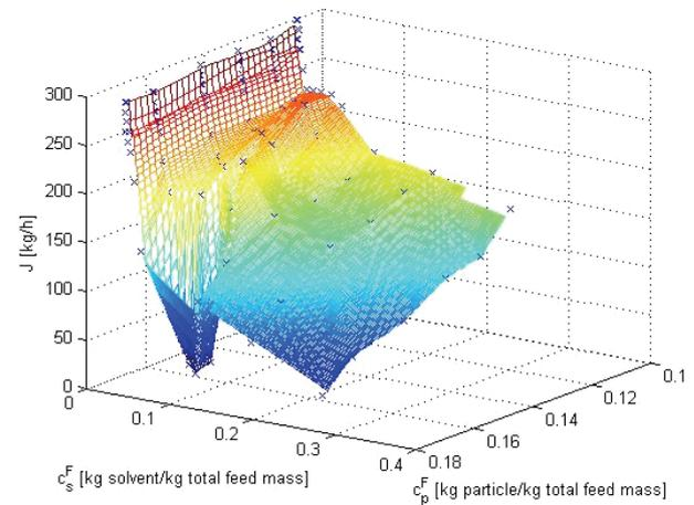
Figure 3: Experimental data of permeate flux (illustrated with x) in the function of particle and solvent concentration (Lines are to guide eyes.)
