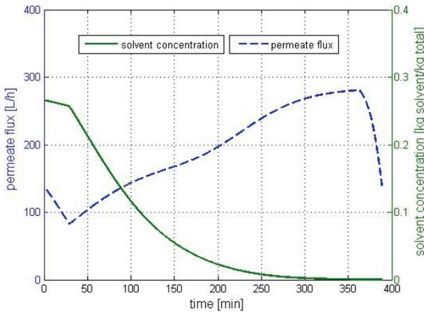
Figure 5: Simulation example for a three-step process including pre-concentration, dilution mode, and post-concentration steps
