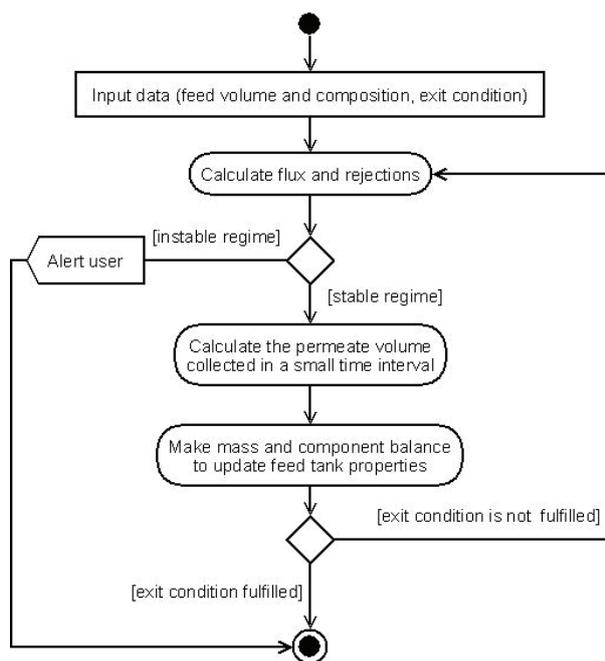
*Figure 2*: UML activity diagram of the process simulation
