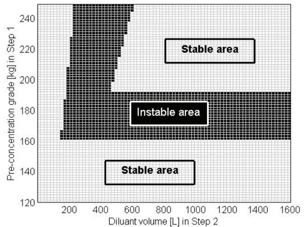
Figure 6: Instable dispersion area illustrated for the applied operational parameters
