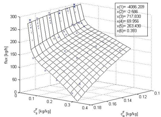
Figure 4: Estimated (solid lines) and experimental data (\*) of permeate flux in the function of solvent and particle concentration (Curve-fitting is based on non-zero flux data.)
