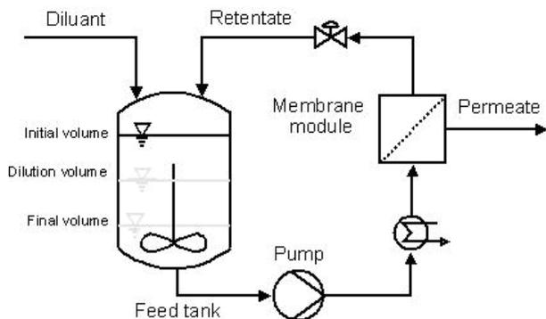
*Figure 1*: Schematic representation of the batch configuration
