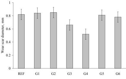
Figure 3: Antiwear properties of the experimental engine oils
