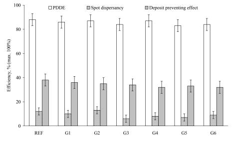
Figure 1: DD and high temperature deposit preventing effects of the experimental engine oils
