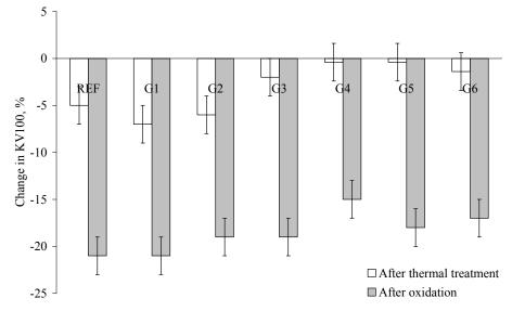
Figure 2: Thermal and oxidation stability of the experimental engine oils
