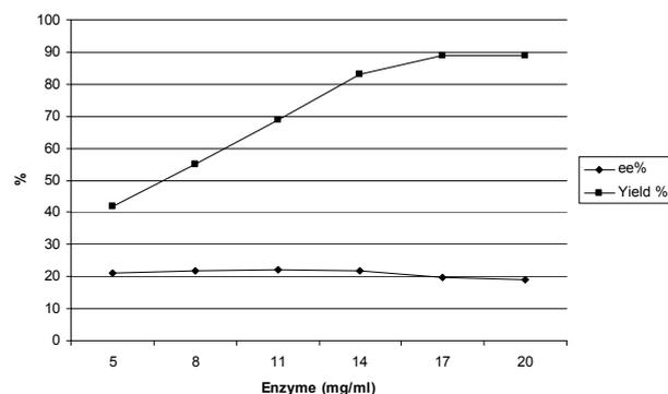
Figure 4 : Effect of enzyme concentration on the enzymatic esterification of lactic acid by ethanol
