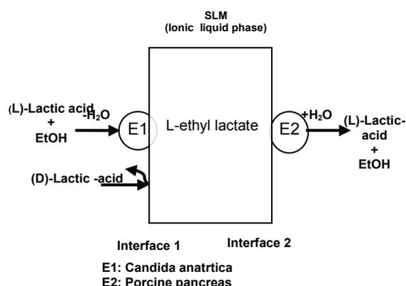
Figure 7: Schematic diagram of enantioselective transport of (L)-lactic acid through a lipase-facilitated SLM based on an ionic liquid
