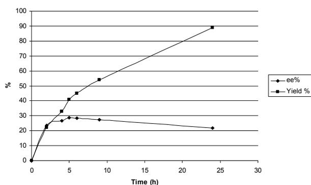
Figure 6: A time course of the esterification between lactic acid and ethanol by Novozymes 435
