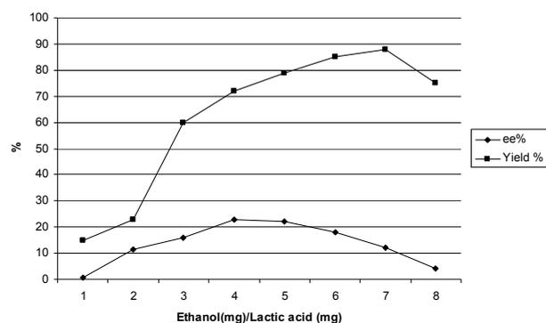
Figure 2: Effect of the molar ratio of alcohol to lactic acid on enantioselectivity of esterification of racemic lactic acid with ethanol, catalyzed by *Candida antarctica*
