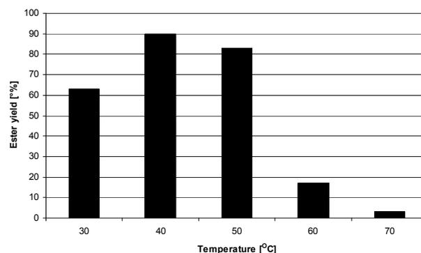
Figure 3: Effect of temperature on the relative value of esterification activity of immobilized lipase
