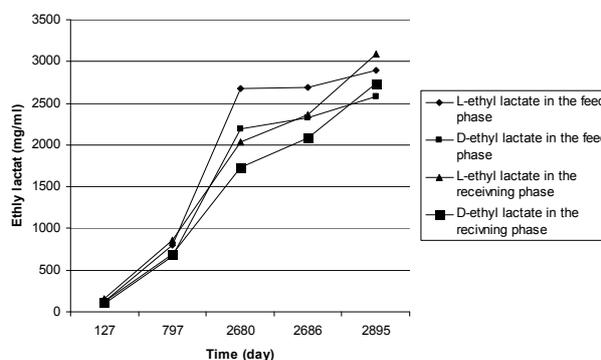
Figure 8: Lipase-facilitated transport of lactic acid through the SLM based on trihexyltetradecylphosphonium bromide
