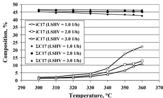
Figure 4: Composition of the  $C_{17}$  fraction as a function of the temperature and the LHSV ( $p = 40$  bar)
