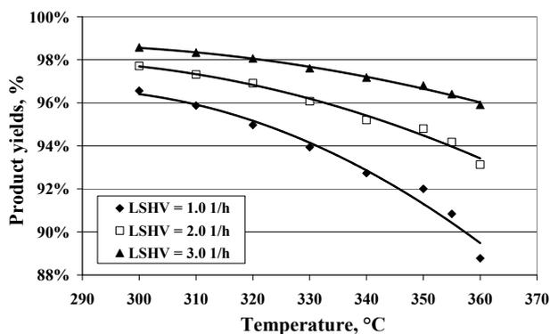
Figure 1: Product yields as a function of the temperature and the LHSV ( $p = 40$  bar)
