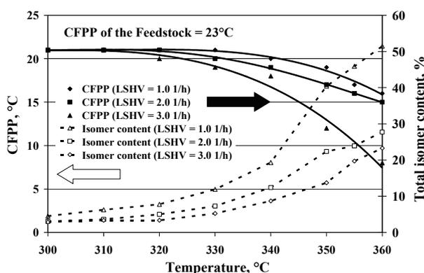
Figure 7: Total isoparaffin content and the CFPP value of the products as a function of the temperature and the LHSV ( $p = 40$  bar)
