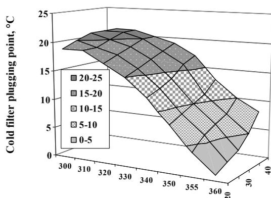
Figure 6: CFPP values of the products as a function of the temperature and the pressure (LHSV = 1.0 1/h)
