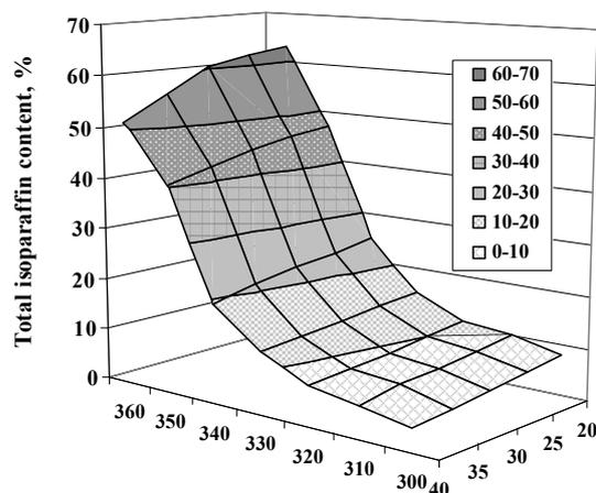
Figure 5: Total isoparaffin content of the products as a function of the temperature and the pressure (LHSV = 1.0 1/h)
