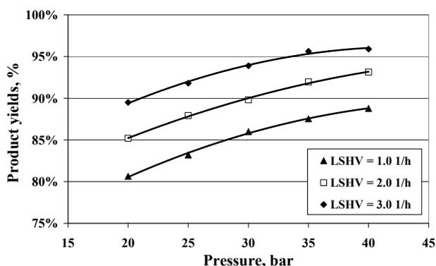
Figure 2: Product yields as a function of the pressure and the LHSV ( $T = 360$  °C)
