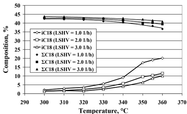
Figure 3: Composition of the  $C_{18}$  fraction as a function of the temperature and the LHSV ( $p = 40$  bar)
