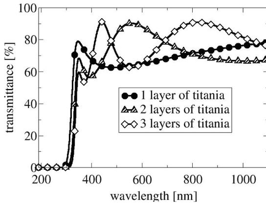
Figure 8: Transmittance spectra of TiO<sub>2</sub> films containing 1, 2 and 3 layers
