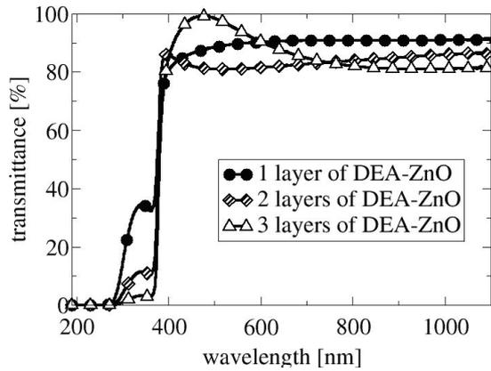
Figure 5: Transmittance spectra of DEA-ZnO films containing 1, 2 and 3 layers
