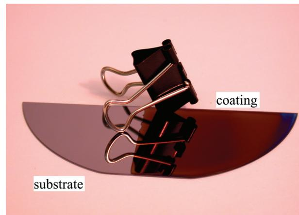
Figure 1: Smooth and reflective surface of TiO<sub>2</sub> film on a piece of 3" Si wafer
