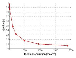
*Figure 2:* Rejection of the membrane Desal-DK5 for NaCl as a function of feed concentration (30 bar, 25 °C, 0.55 m<sup>2</sup> spiral-wound element, 1.0 m<sup>3</sup>h<sup>-1</sup> recirculation flow-rate). Solid line is for eye guidance
