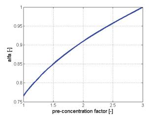
*Figure 4:* Optimized α values as a function of preconcentration factor for the PVVD process
