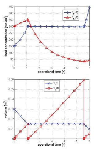
*Figure 3:* The estimated 6-hour time-course of the concentrations and the volumes of feed and permeate for a traditional diafiltration process with a preconcentration-factor of 2
