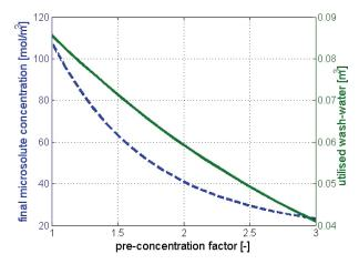
*Figure 5:* Optimization diagram for traditional diafiltration. Final microsolute concentration (dashed line) and required wash-water volume (continuous line) are plotted versus pre-concentration factor
