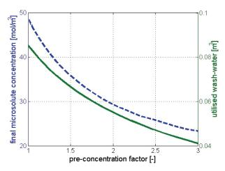
*Figure 6:* Optimization diagram for diafiltration involving pre-concentration combined variable-volume dilution. Final microsolute concentration (dashed line) and required wash-water volume (continuous line) are plotted versus pre-concentration factor
