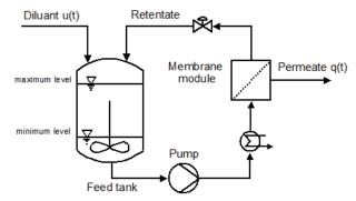
Figure 1: Schematic representation of diafiltration settings
