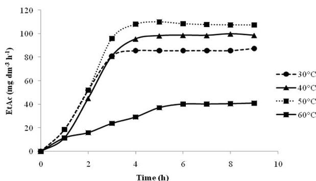
Figure 4: Effect of temperature on ethyl-acetate yield as a function of time
