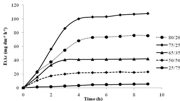
Figure 6: Effect of initial substrate composition on ethyl-acetate yield as a function of time
