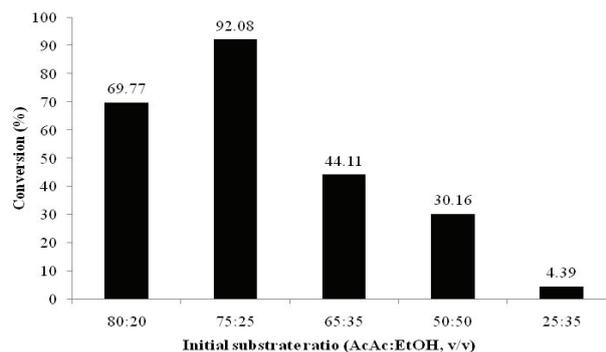
Figure 7: Effect of initial substrate composition on acetic acid conversion
