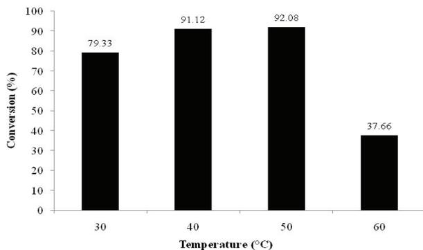
Figure 5: Effect of temperature on acetic acid conversion
