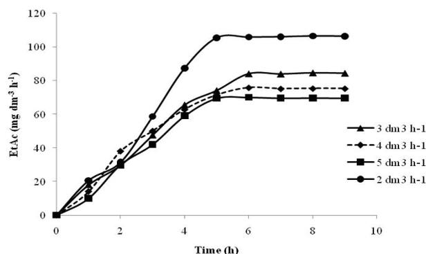
Figure 2: Effect of carrier gas flow rate on ethyl-acetate yield as a function of time
