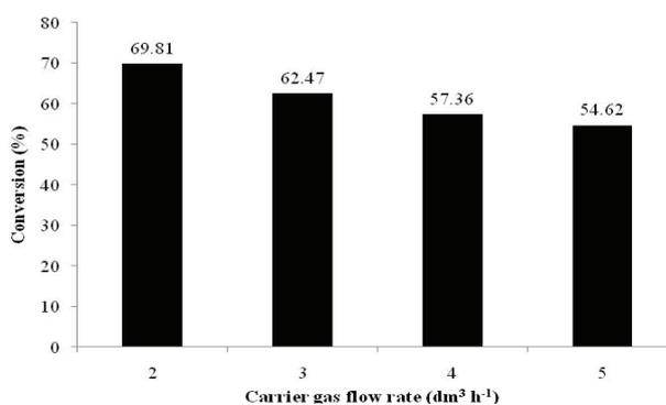
Figure 3: Effect of carrier gas flow rate on acetic acid conversion
