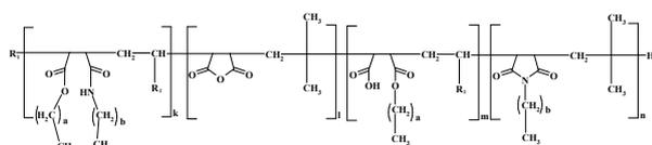
**Figure 1:** Structure of the ester-amide-imide derivative of the experimental olefin-maleic-anhydride copolymer (R1: alkyl group with length of the olefinic monomer (C16-C18); R2: alkyl group with R1-2 carbon number; a: 3-40, b: 3-32; k: 0,2-2; l: 1-7; m: 1-7 and n: 0,3-2)
