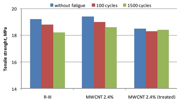
Figure 9: Effects of surface treatment on fatigue tensile properties (fatigue load: 10 N)
