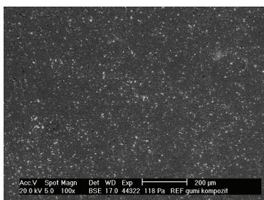
Figure 12: SEM graph of the broken surface of the original rubber matrix
