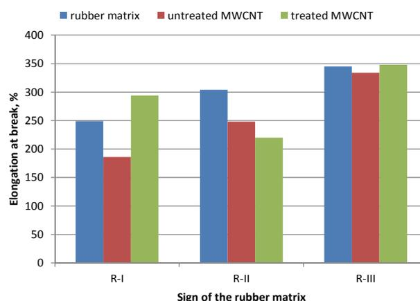
Figure 4: Effects of type of the rubber matrix on elongation at break (1 wt% MWCNT content)
