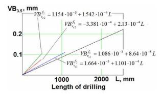
*Figure 10:* The changes of the flank wear in cutting speed and feed rate depending on dry machining
