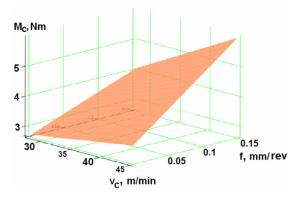
*Figure 6:* The changes of the torque in cutting speed and feed rate depending on dry machining with sharp tool
