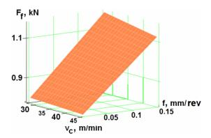
*Figure 5:* The changes of the thrust in cutting speed and feed rate depending on dry machining with sharp tool
