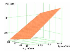
*Figure 7:* The changes of the average surface roughness in cutting speed and feed rate depending on dry machining with sharp tool
