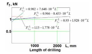
*Figure 8:* The changes of the thrust in cutting speed and feed rate depending on dry machining
