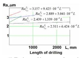
*Figure 12:* The changes of the average surface roughness in cutting speed and feed rate depending on dry machining
