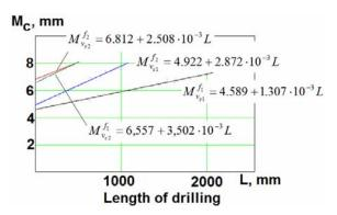
*Figure 9:* The changes of the torque in cutting speed and feed rate depending on dry machining
