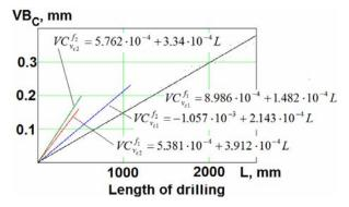
Figure 11: The changes of the corner wear in cutting speed and feed rate depending on dry machining
