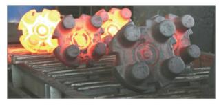
Figure 11: Planetary carriers on BY equipment
