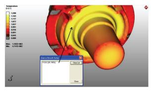
*Figure 3:* Surface temperature is 1133 °C at a properly measurable location
