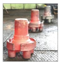
*Figure 6*: Planetary carriers cooled in quiet air, without air flow
