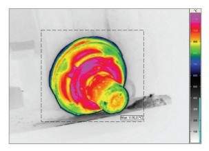
*Figure 4:* Photo taken with thermographic camera. Emission factor: 0.95
