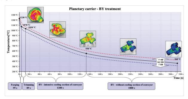
Figure 10: Cooling diagram of planetary carrier
