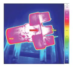
*Figure 7:* Photo taken by thermographic camera on start of intensive cooling stage. Emission factor: 0.95
