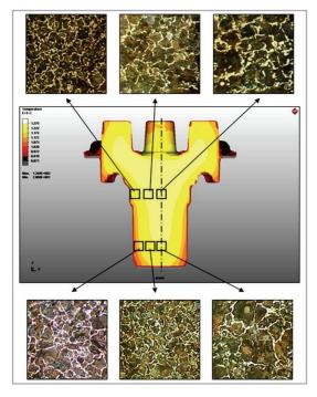
*Figure 9*: Relationship between the internal heat distribution and the microstructure
