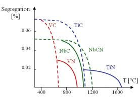
Figure 1: Example for segregation of micro-alloys
