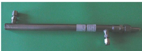
Figure 1: The capillary membrane module
