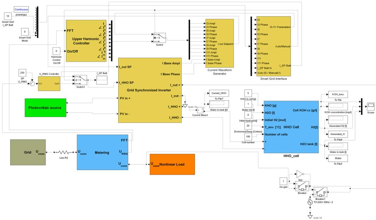
Figure 7: Simulink model of a complex energetic system with an HHO cell model inside
