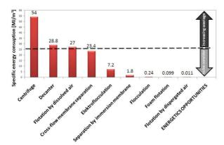
*Figure 4*: The energetic consideration of selected separation processes (the dashed line shows the energy content of algae suspensions on average of 25 MJ m<sup>-3</sup>)
