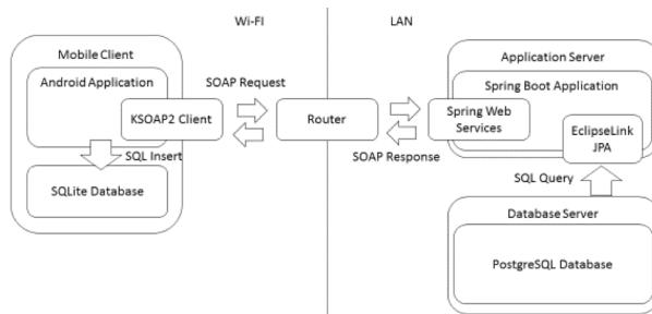
Figure 2. The SOAP based test application's logical architecture. The communication between the client and server component is based on XML / SOAP messages.
