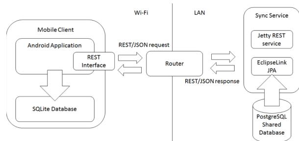
Figure 3. The REST based test application's logical architecture. The communication between the client and server component is based on JSON / REST messages.
