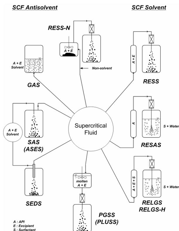
Fig. 1 Schematic diagram of supercritical particle engineering technologies.
