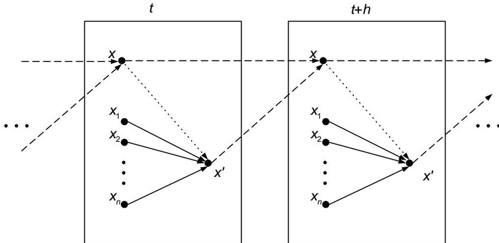
Fig.1 Dynamic representation graph assuming first order explicit solution method
