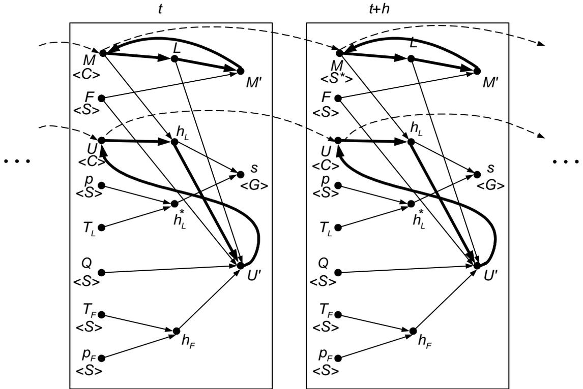
Fig.11 Representation graph of model  $M_1$  with Specification 1 assuming an implicit solution method ( $\rightarrow$  circle of calculation)
