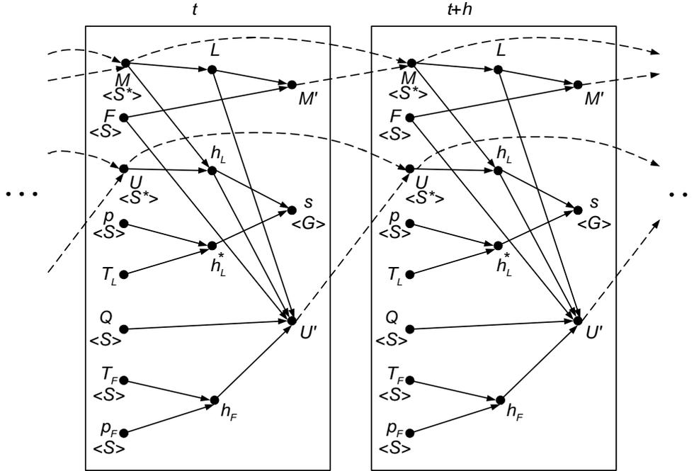
Fig.2 Representation graph of model  $M_1$  with Specification 1 assuming first order explicit method
