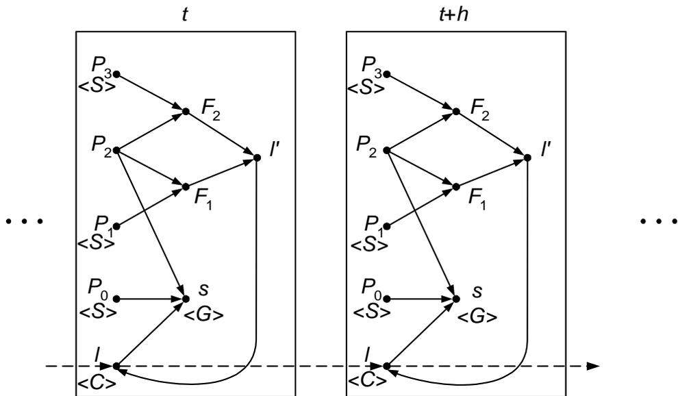
Fig.12 Representation graph of model  $M_2$  assuming an implicit solution method
