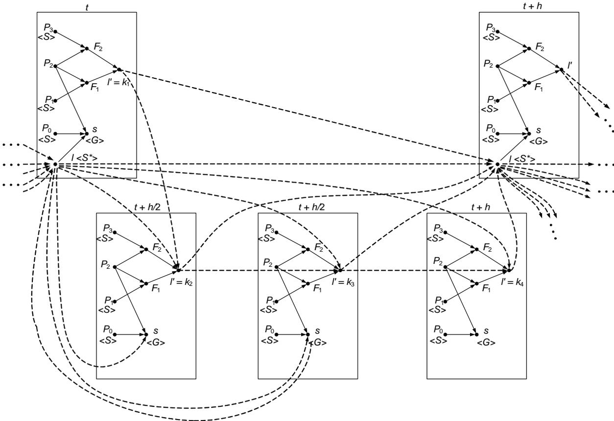
Fig.9 Representation graph of model  $M_2$  assuming fourth order explicit Runge-Kutta method
