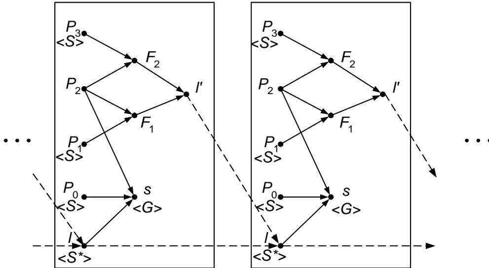
Fig.6 Representation graph of model  $M_2$  assuming first order explicit solution method
