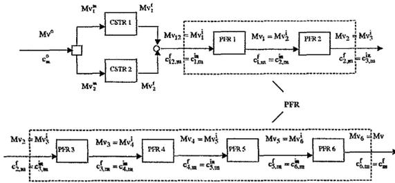
Fig. 1 Reactor network for polystyrene production by bulk polymerisation
