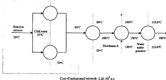
Fig.2 Optimal heat exchanger network for polystyrene manufacturing by bulk polymerisation
