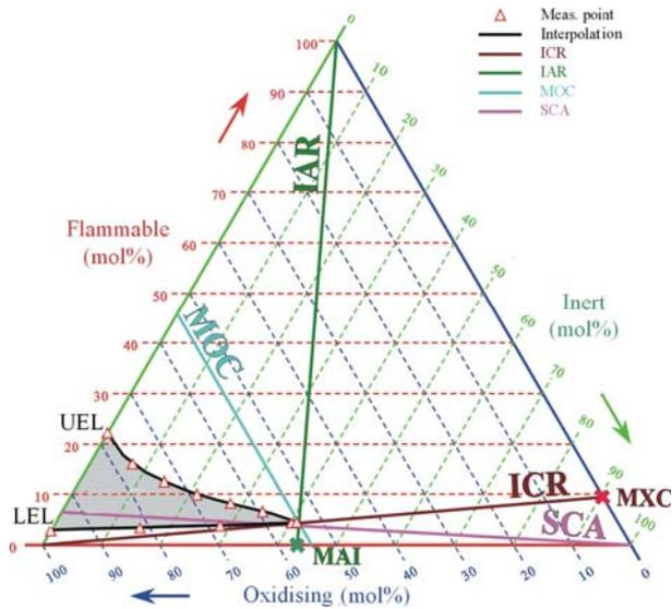
Fig. 1: Characteristics of the explosion area
