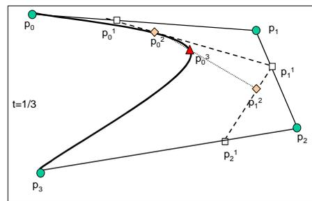
Fig. 2.: The four frame points of a co-monotonic spline and evaluating  $p_0^3$  at  $t=1/3$
