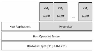
Fig. 2. Typical Virtual Machine architecture [1].
