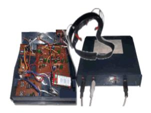
Fig. 3. EEG hardware unit to capture EOG signals.
