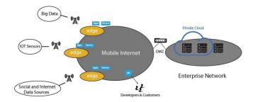
Fig. 7: Mobile edge computing architecture [68].
