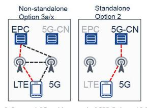
Fig. 5: Proposed 5G architectures in 3GPP Release 15 [31].
