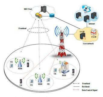
Fig. 6: Schematic of C-RAN architecture [65].
