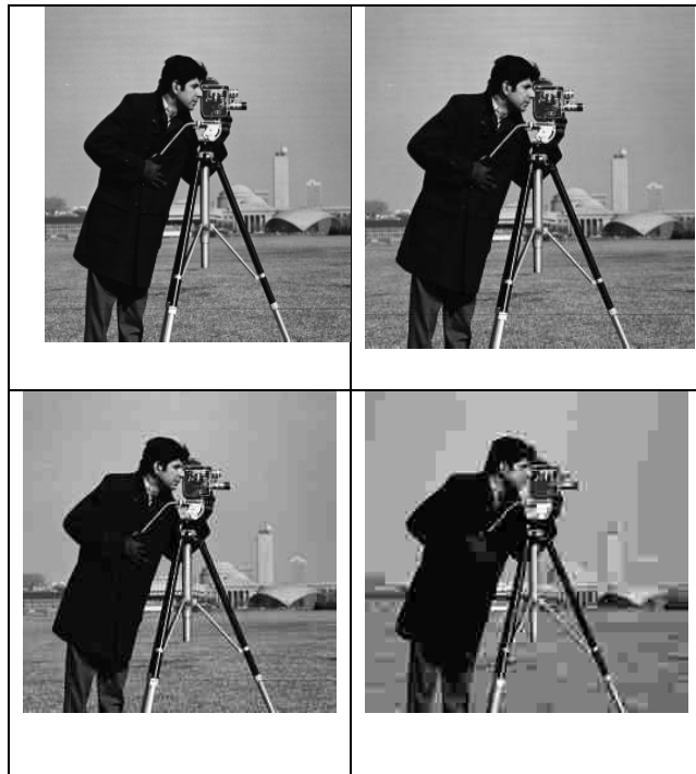
Fig. 11: Simulation results using Standard JPEG. (a) Original test image (top left). (b) Compression ratio 8:1, PSNR=33.19 dB (top right). (c) Compression ratio 32:1, PSNR=24.3 dB (bottom left). (d) Compression ratio 64:1, PSNR=16.9 dB (bottom right).
