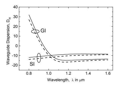
Fig. 10: Effect of the ocean depth (from 0 to 3 km) on the waveguide dispersion parameters as a function of the wavelength for the step index (SI) and graded index (GI) fibers
