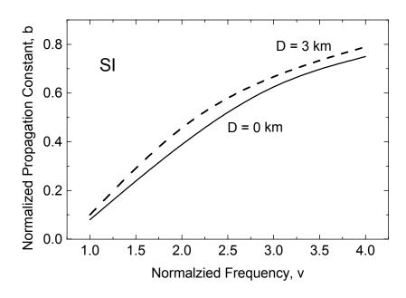
Fig. 3: The variation of the propagation constant with the normalized frequency at 0 and 3 km depths for the step index fibers
