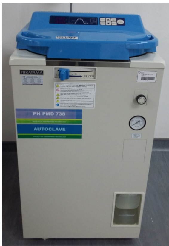
Fig. 1: Autoclave machine used to synthesize AgNPs at 121^\circ\text{C} for 20 minutes.
