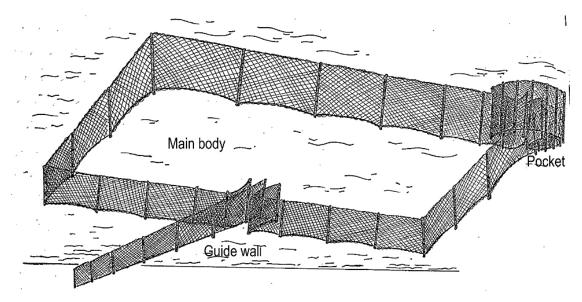
Figure 1. Schematic drawing of a Moshta showing its three main parts.
