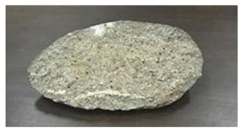
Figure 31. Lumashell, Khamir Port breakwater (Photographed by Zohreh Moradi).
