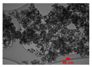
Figure 1. TEM micrographs of the Nano-ZnO powders (Adapted from Iranian Nano-materials Pioneers Company's catalog).
