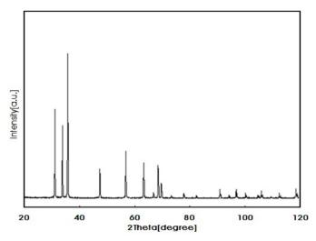
Figure 3. The X-ray powder diffraction (XRD) curves of Nanocrystalline ZnO (Adapted from Iranian Nano-materials Pioneers Company's catalog).
