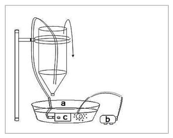
Figure 1. Schematic design of the semi-closed incubator: a, collector vessel; b, aeration pump; c, water recirculation pump.
